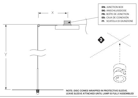
PROVIDED LAMP WIRES ARE 8', LAMP HANG HEIGHT REDUCES IN RELATION TO SWAG DISTANCE FROM CANOPY. IF X=5', Y CAN BE A MAXIMUM OF 3'.
